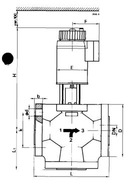
Flange dimensions according to DIN 2533, PN16
