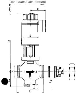
In the case of the screwed valves, screwed fittings are supplied.
